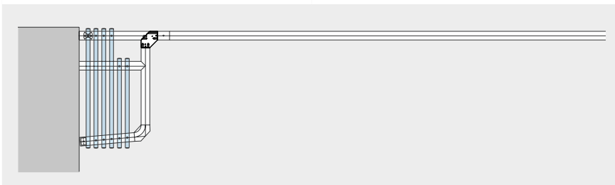
Stacking panels of varying width.
